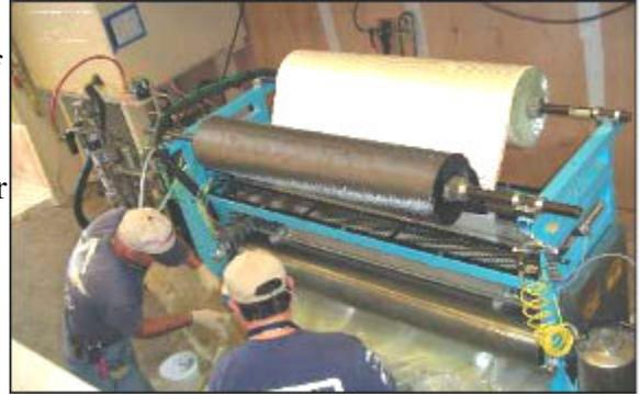
An impregnator supplies and uniformly regulates the resin to fiber ratio of composite laminates.
